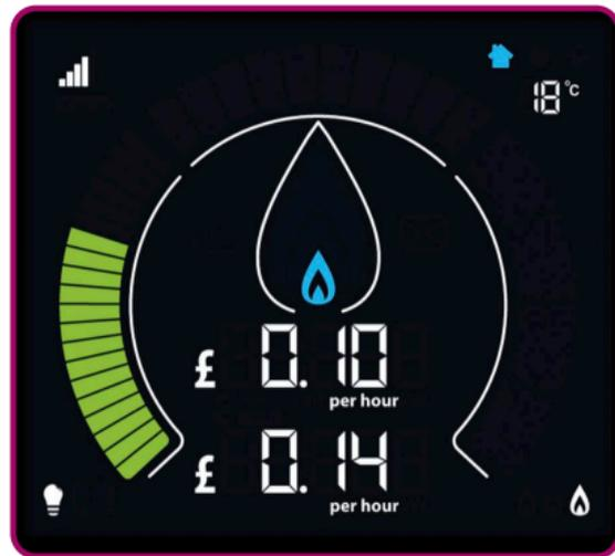
Your current usage is displayed on the left hand side of the Home screen. The outer gauge shows your electricity, and the inner flame your gas. You can use the touch-sensitive unit selectors to view your usage in pounds and pence, kilowatt hours (kWh) or carbon emissions.
