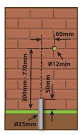
A 12mm hole is required to link the external Network to the internal one.
