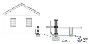
Fig 1: Indication of backflow into a water main.
