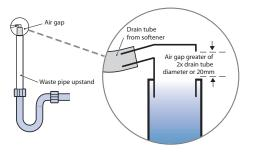
Fig 3: Connection to drainage system via an air gap
