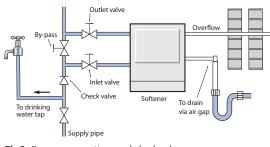
Fig 2: Bypass, connections and check valve
