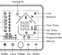
**1. Power On/off:** Press O to turn the thermostat on/off.
