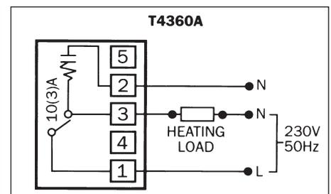
N.B. Contact closes when temperature falls below the thermostat setting
