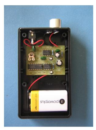
The enclosed instruction leaflet advises that several resistors can be tried for the R2 position however; using the above components from Rapid the 0.6w 1K resistor M1K will work adequately.
